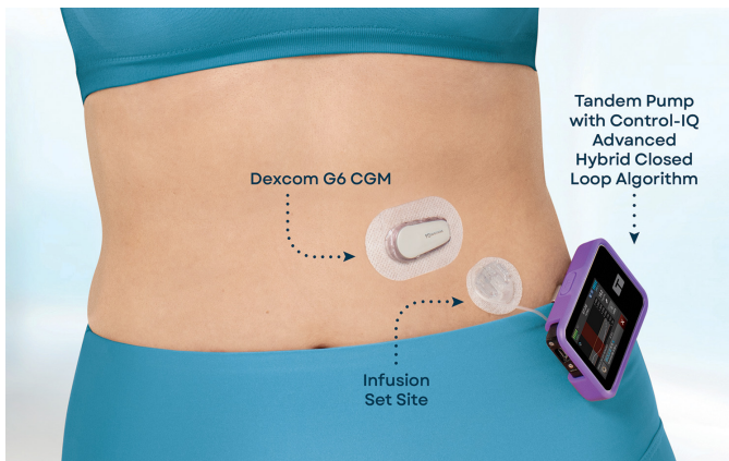
Figure 1: The image shows how an individual usually wears a HCL system (i.e., a CGM along with an insulin pump with an algorithm). The CGM senses glucose levels and sends data to the insulin pump via Bluetooth. The insulin pump shows glucose numbers and predicted trends and delivers insulin to the body. The algorithm embedded in the insulin pump predicts glucose levels and adjusts insulin delivery accordingly.
