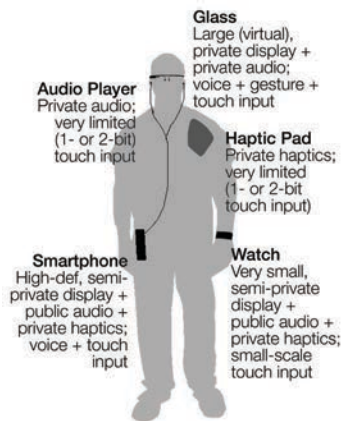
Figure 3. Devices that are part of the contemporary/emerging wearable display ecology for personal informatics.
