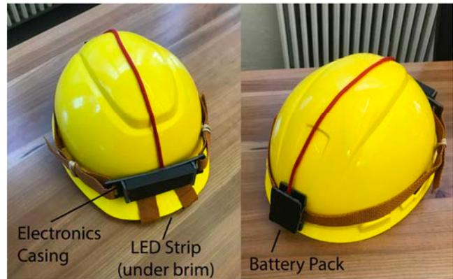
Figure 1: Physical prototype representing the design of a proposed helmet-mounted visual peripheral navigation aide.
