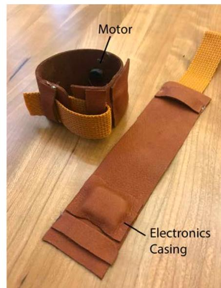
Figure 2: Physical prototype representing the design of a proposed pair of arm-worn haptic peripheral navigation aides.
