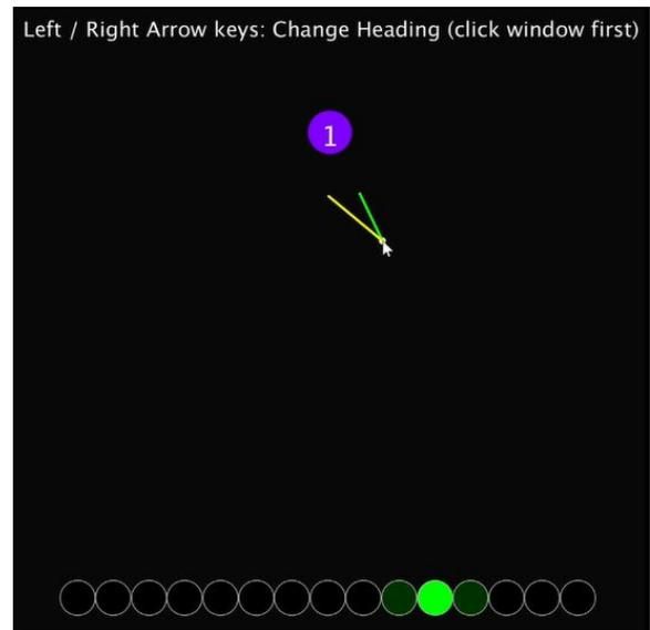
Figure 4: The interactive graphical prototype. The yellow line represents the direction a user is facing, the green line represents the azimuth, and the row of circles represents the LED display
