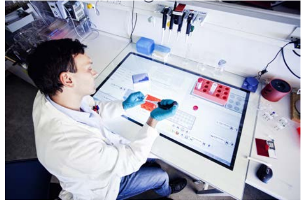
Figure 7: The electronic laboratory workbench (eLabBench) (from [21]).
