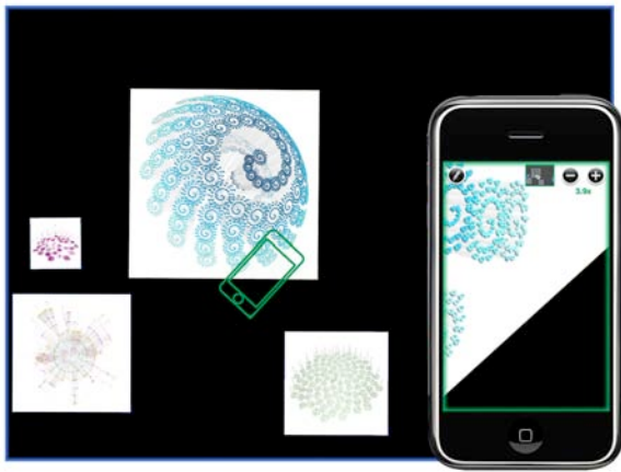
Figure 6. The iPodLoupe lens, overlaid on a tabletop displaying several PhylloTree visualizations [24]. Although similar to the i-Loupe in function and design, iPodLoupe differs in two ways: (1) the focus component exists only on the handheld, and (2) the iPod enables gestural, multi-touch input.
