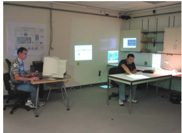
Figure 2. An overview of the experimental setup (prior to installing the “round table”). The “wizard” is seated at his control station on the left, and a researcher is playing the role of a participant on the right. Note the projected images on the wall, desk, and floor surfaces.
