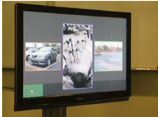
Fig. 5. An inSpace Wall, displaying artifacts shared by three meeting participants. The meeting participant represented by the green color is currently uploading a new file to the Wall, indicated by the status bar display at the lower left.
